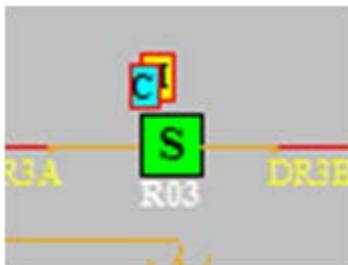
Figure 3: HMI breaker close up, caution & hold cards applied
